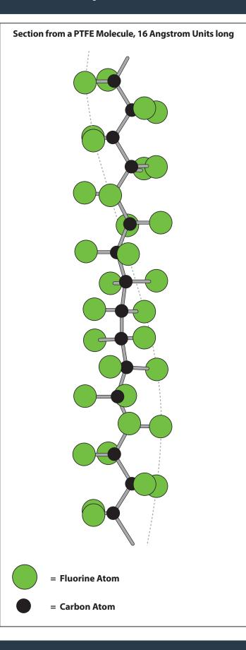
PTFE, or Polytetrafluoroethylene, comprises of longchain molecules of carbon atoms, each linked to two fluorine atoms.
