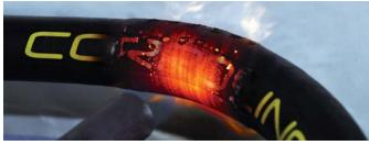
Corroline<sup>+</sup> GP and AS grade hose is Fireproof to BS5173 Section 103.13 Part 6.2 and 6.3. When end fittings are assembled to the hose, the assembly is Fire Resistant, but can be made Fireproof by adding DBK-300 rubber cover end protection. Corroline<sup>+</sup> meets the requirements of German safety regulation TRbF 131/2 and EN 16643 flame resistance.
