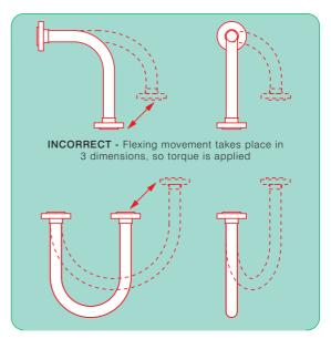
Both Corroflon and Bioflex hose have good resistance to a small level of torque, much better resistance that rubber or SS hose types, but it is still the best practice to take whatever steps are necessary to eliminate torque. If in doubt, consult Aflex Hose.
